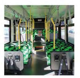
New composite flooring, lightweight seating, and LED interior/exterior lighting is installed.
