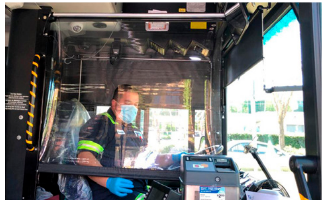
Employees at VTA in Santa Clara, CA make barriers out of decommissioned bus parts. Source: vta.org 10
